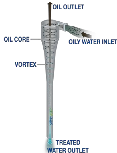
Figure 1.1.2: Schema showing centrifugal forces in a hydrocyclone for oily water separation
