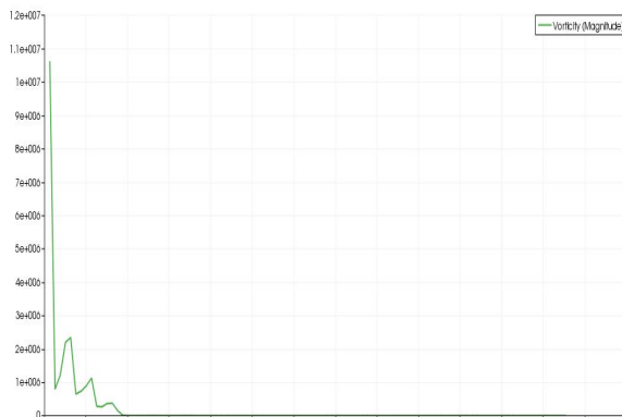
Curve showing the evolution of the vorticity in turbulent regime (in s^{-1} )
