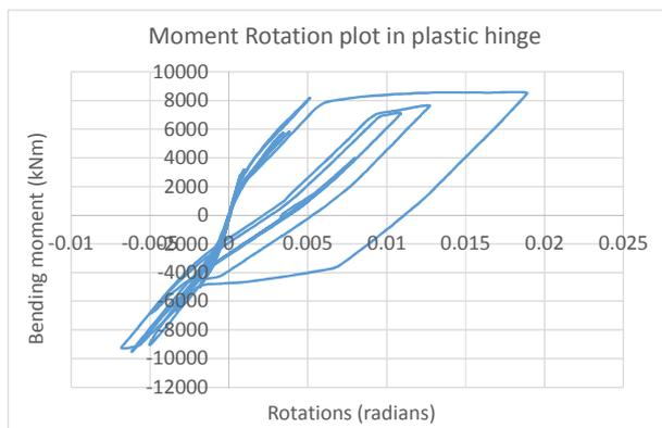
Fig. 8. Moment rotation diagram in plastic hinge from non-linear time history analysis
