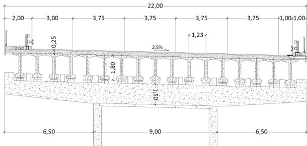
Figure 1. Cross section of the original design
