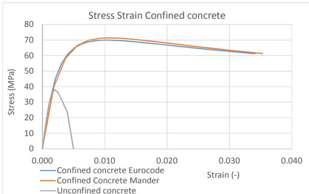
Fig. 6: stress strain relationship for concrete
