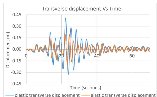
Figure 7. Transverse displacement of the deck above pier 6 Vs time
