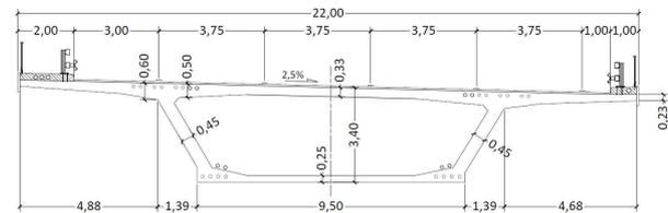
Figure 4. Typical cross section
