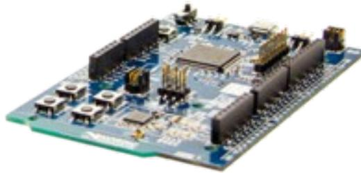
figure 10: nRF51 DK (Nordic Semiconductor)
