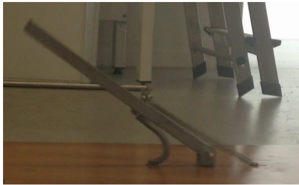
FIGURE 4.5 – Photo illustrant le flambage du ressort
