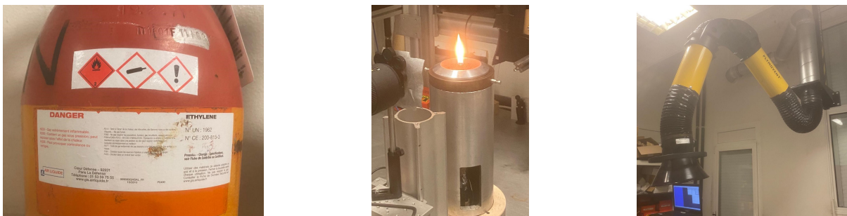
Figure 2: Images of the ethylene bottle, the Gulber Burner and the exhaust
