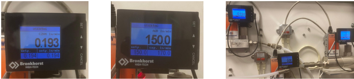
Figure 1: Images of the air and ethylene mass flow controllers
