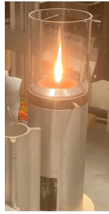
Figure 4: Image of the Burner and the added tube
