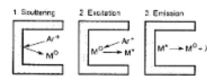
The workings of a hollow cathode lamp (HCL).
