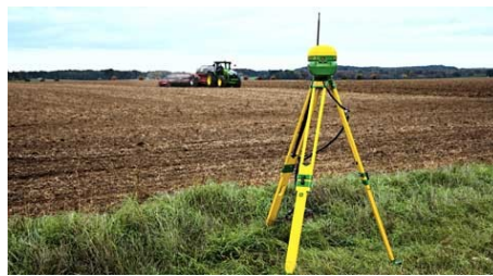
Figure 6: Base fixe d'un GPS RTK https://www.fwi.co.uk/machinery/a-guide-to-guidance-part-3-rtk
