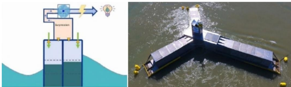
Figure 11 : HACE multi chambre offshore system [11]
