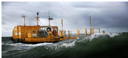
Figure 9 : Ocean Energy buoy with Wells turbine [9]
