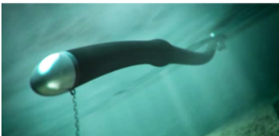
Figure 19 : The Anaconda wave energy converter [19]
