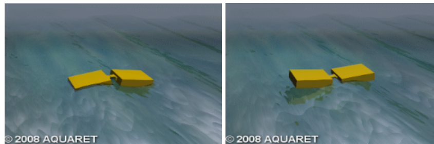
Figure 16 : Principle of operation of an attenuator [16]
