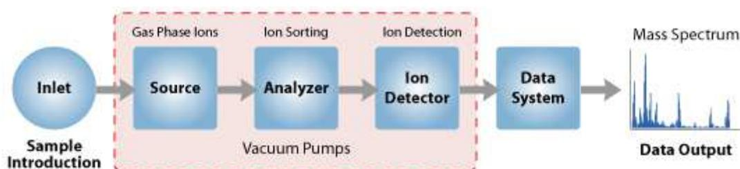
Figure 1 : Principle of spectrometer
