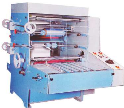
Figure 8 : Machine appliquant la technique LOM
