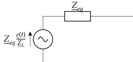
On trouve  $e_{th}(t) = \underline{Z}_{eq} \frac{e(t)}{\underline{Z}_L} = \frac{\underline{Z}_C}{\underline{Z}_L + \underline{Z}_C} e(t)$  et  $\underline{Z}_{th} = \underline{Z}_{eq} = \frac{\underline{Z}_L \underline{Z}_C}{\underline{Z}_L + \underline{Z}_C}$ .
